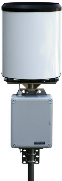
Thalassa-H1 cabinet installed on SR03 rainfall gauge stand
